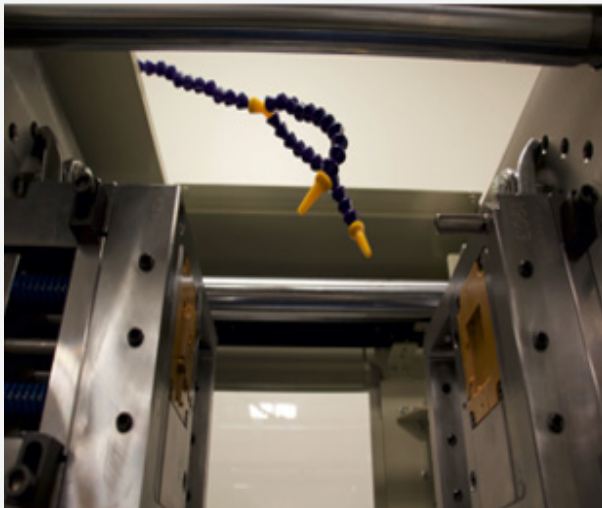
FIGURE 8. Nozzle blowing compressed air on 3D printed mold tool
